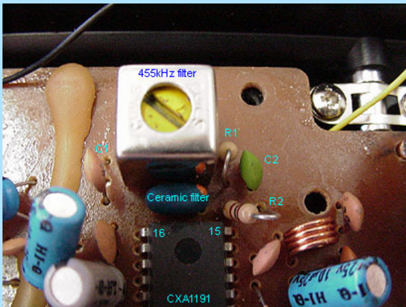
Top layer of the 455kHz IF transformer and the ceramic 10.7MHz filter
